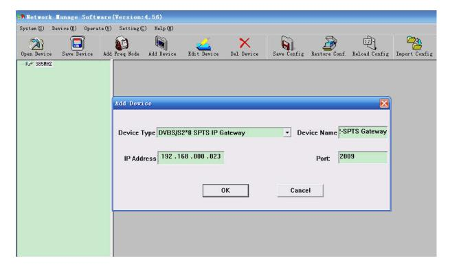
Choose device type" \*\*\*\*\*\*\*, set device name (you can name as you like), and set IP address and Port of the device. You can check IP address by clicking down key on the panel or you can enter into "Network Setting" in the menu to check it. Default IP address and Port are 192.168.000.023 and 2009.
